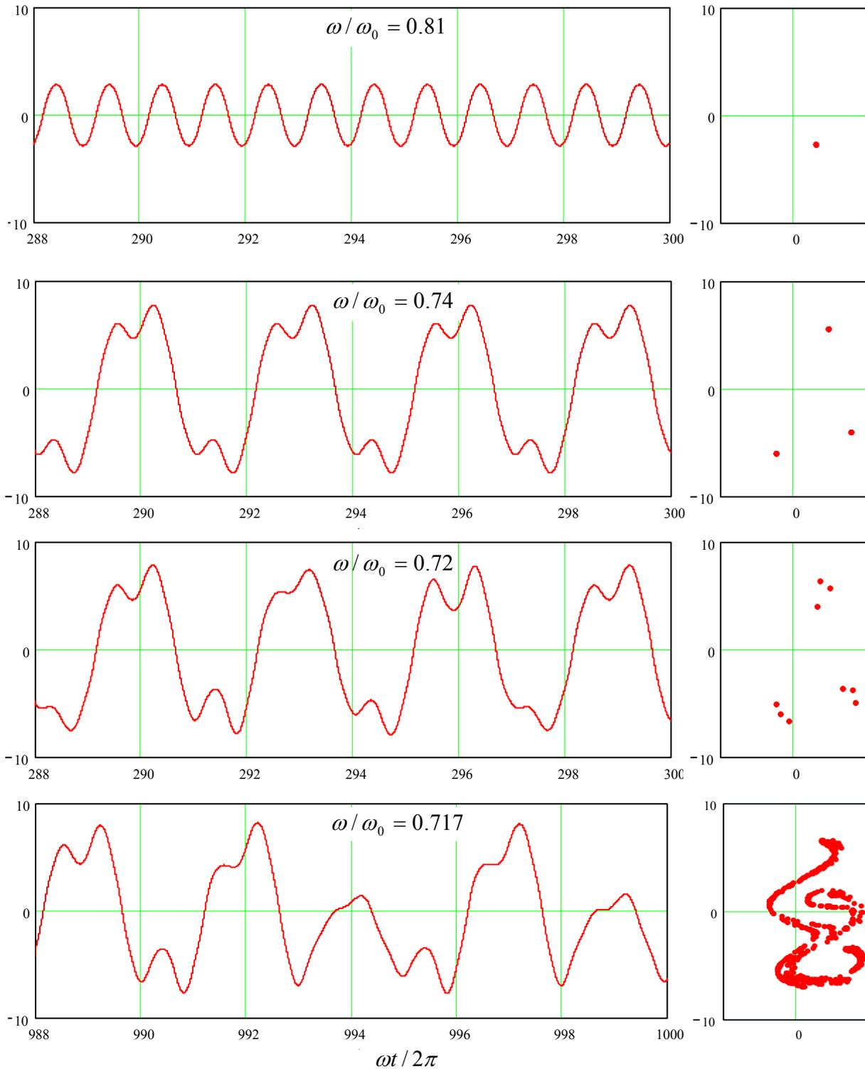
Fig. 9.4. Oscillations in a pendulum with weak damping,  $\delta/\omega_0 = 0.1$ , driven by a sinusoidal external force with a fixed effective amplitude  $f_0/\omega_0^2 = 1$ , and several close values of the frequency (listed on the panels). Left column: oscillation waveforms  $q(t)$  recorded after certain initial transient intervals. Right column: representations of the same processes on the Poincaré plane of variables  $[p, q]$ .
