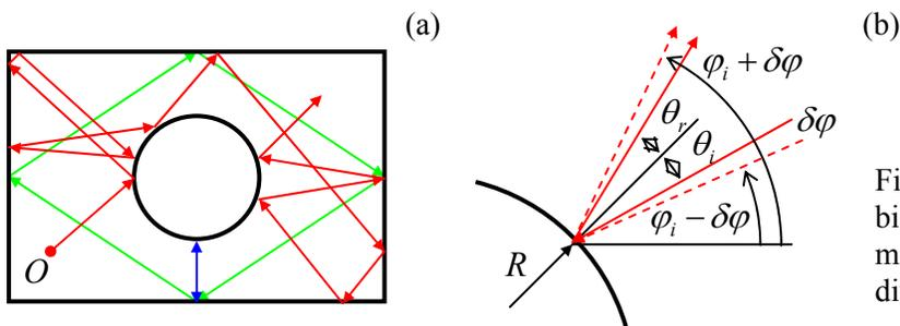
Fig. 9.8. (a) Motion on a Sinai billiard table, and (b) the mechanism of the exponential divergence of close trajectories.
