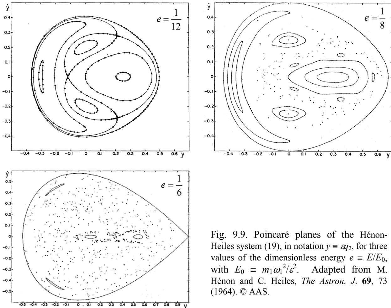
Fig. 9.9. Poincaré planes of the Hénon-Heiles system (19), in notation  $y \equiv \varepsilon q_2$ , for three values of the dimensionless energy  $e \equiv E/E_0$ , with  $E_0 \equiv m_1 \omega_1^2 / \varepsilon^2$ . Adapted from M. Hénon and C. Heiles, *The Astron. J.* **69**, 73 (1964). © AAS.
