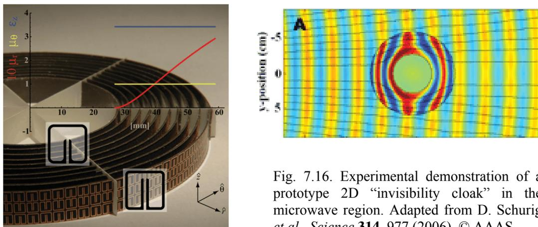
Fig. 7.16. Experimental demonstration of a prototype 2D “invisibility cloak” in the microwave region. Adapted from D. Schurig *et al.*, *Science* **314**, 977 (2006). © AAAS.
