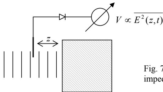
Fig. 7.9. Measurement of the complex impedance of a medium (schematically).
