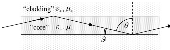
Fig. 7.25. Wave propagation in a thick optical fiber.
