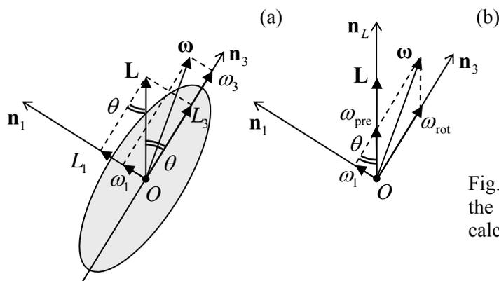
Fig. 6.9. Free rotation of a symmetric top: (a) the general configuration of vectors, and (b) calculating the free precession frequency.
