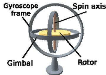
Fig. 6.8. Typical gyroscope. (Adapted from <http://en.wikipedia.org/wiki/Gyroscope>.)
