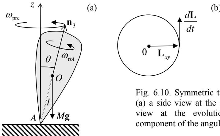
Fig. 6.10. Symmetric top in the gravity field: (a) a side view at the system and (b) the top view at the evolution of the horizontal component of the angular momentum vector.
