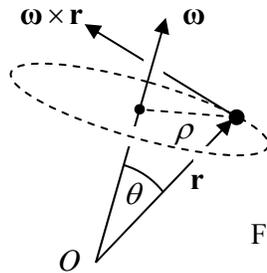
Fig. 6.2. Instantaneous axis of rotation.
