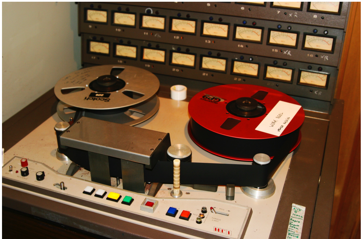
Figure 3: Two-inch tape machine at Eastern Bloc Studios, Melbourne, Victoria, March 28, 2006. DAW interfaces were initially designed around the functionality of physical machines using the analogy of tape transport controls. In some studios, DAW systems are still used alongside tape machines, although modern workflows often contain production completely within the digital realm. Photo by author.
