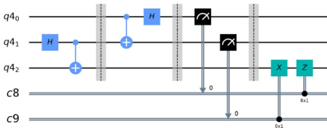
**Figure 3:** Teleportation quantum circuit (Adapted from Asfaw et al., *Learn Quantum Computation Using Qiskit*, 2020, Section 3.2 Quantum Teleportation)
